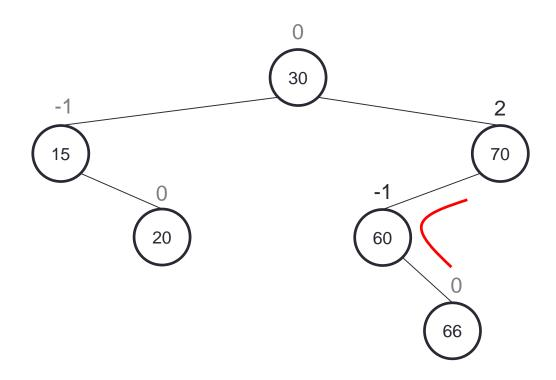
Single rotations only work to balance the tree when involved nodes are "in a line" This is not the case here. We want 66 to be the top node, not 60. So we will first rotate left at 60 to get 66 in the middle, then we can rotate right at 70.
