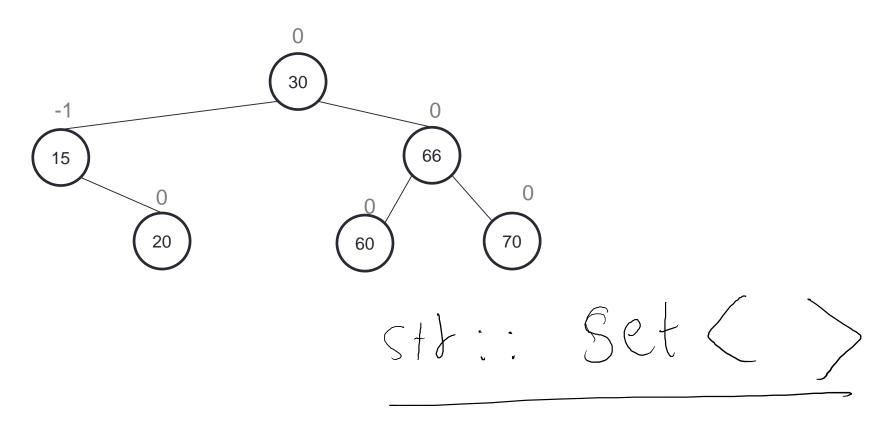
Single rotations only work when involved nodes are "in a line" So we will first rotate left at 60, then we can rotate right at 70.
