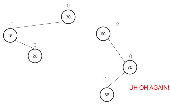
Reattaching 66 here will always work with respect to the BST properties, and we know that 66 will always fit here because 60 used to be 70s left child.
