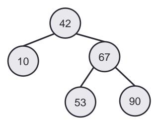
The balance factor at a node in a tree is height(left subtree) – height(right subtree)
