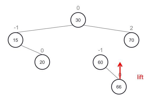
Single rotations only work when involved nodes are "in a line" So we will first rotate left around 60, then we can rotate right around 70.
