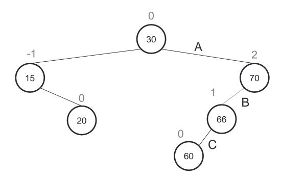
Single rotations only work when involved nodes are "in a line" So we will first rotate left around 60, then we can rotate right around 70.
