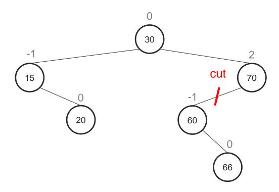
Single rotations only work when involved nodes are "in a line" So we will first rotate left at 60, then we can rotate right at 70.
