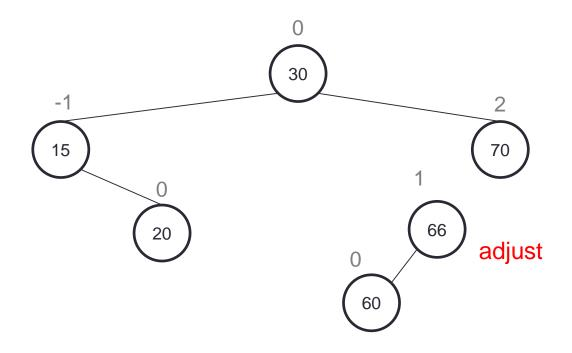
Single rotations only work when involved nodes are "in a line" So we will first rotate left at 60, then we can rotate right at 70.
